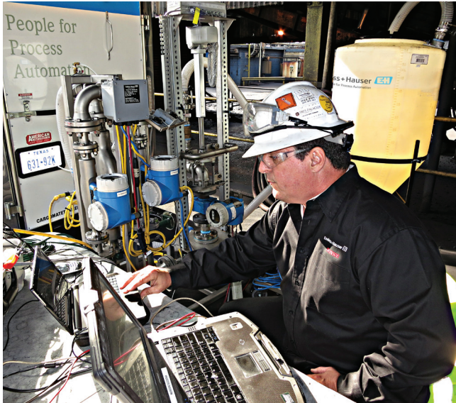
Calibration at customer's site.
